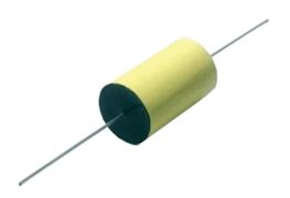
Type 951C, axial leaded metallized polypropylene capacitors are designed for UPS systems and other AC output filtering applications. With integrated fused metallization pattern, this product features UL 810 recognition for fail-safe operation at temperatures up to 85 °C.
